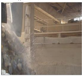
Water spraying System in Crusher Hopper
